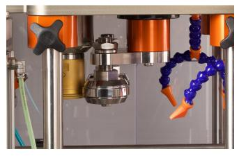
Seaming on the IMP2 is completed effortlessly and accurately due to our revolutionary new electronic seamer. The proven system provides industry standard double seams that can be compared to any high end multi head machines. Microcan have developed seamer tooling with a proven extensive double lifespan. If adjustments are required, they can be carried out simply on screen to maintain high tolerances.
